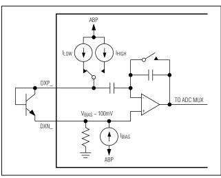
Figure 4. Remote Temperature Sensor Amplifier Circuitry
