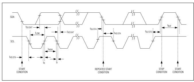
Figure 1. SMBus Interface Timing Diagram
