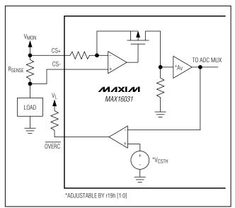
Figure 3. Current-Sense Block Diagram
