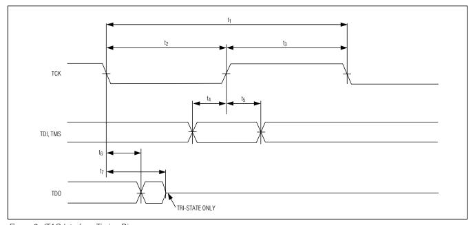
Figure 2. JTAG Interface Timing Diagram
