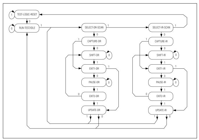
Figure 7. TAP Controller State Diagram
